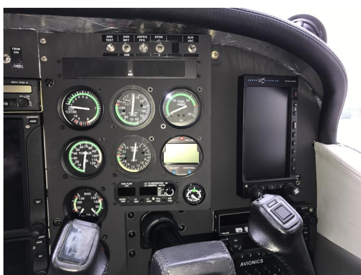
Garmin GTN750 + GNS430W + GTX330 (Engine Instruments now replaced) ASPEN PDF1000
