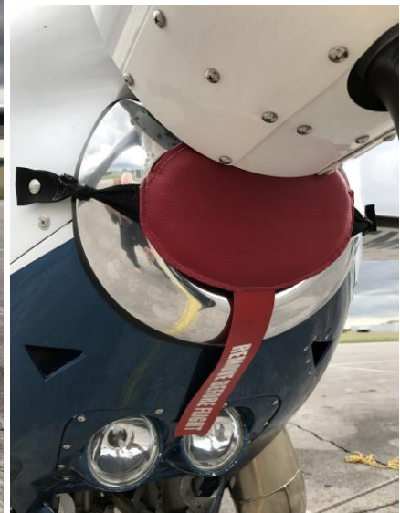
New stainless steel heated air intake New Halogen Landing Lights
