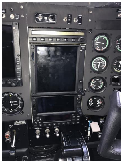
Garmin GTN750 + GNS430W + GTX330 (Engine Instruments now replaced) ASPEN PDF1000
